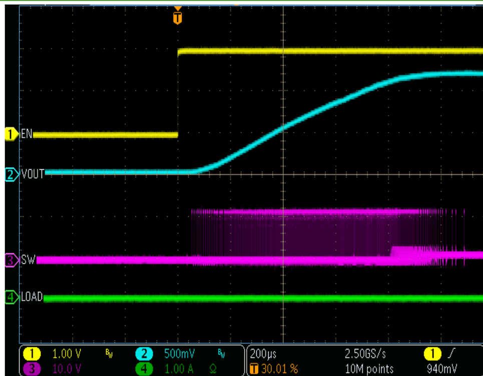
Startup, 12V Vin, 1.2V Vout, No LOAD
